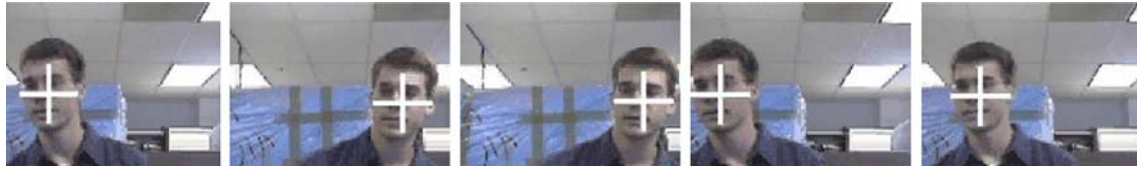
Fig. 18 Frames 1, 8, 12, 20, and 25 of the seq_fast.avi sequence, in which the proposed algorithm tracks the face even during its fast left and right motion. However, the mean-shift and condensation trackers could not track the fast-moving face (see Fig. 6 in [45])
