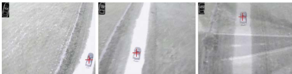
Fig. 17 Frames 1, 100, and 190 of a shaky video sequence recorded from an unmanned aerial vehicle (UAV) showing a small car being tracked perfectly by our algorithm in the presence of blur, glare, and UAV motion in 6 degree-of-freedom
